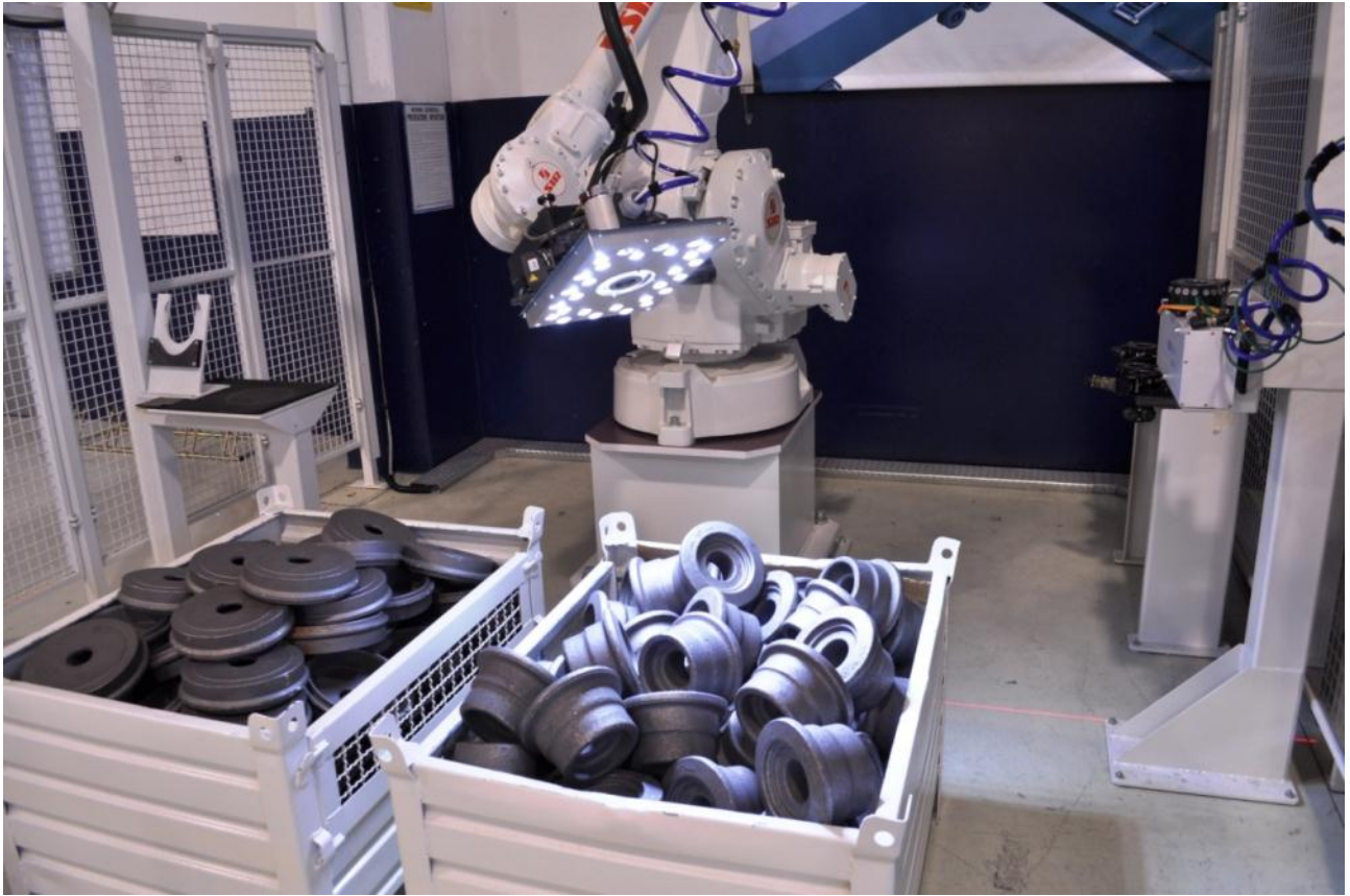
Figure 4 - Robotic system arranged with a stereoscopic vision system (3D) (courtesy: SIR Spa – MO, Italy).
