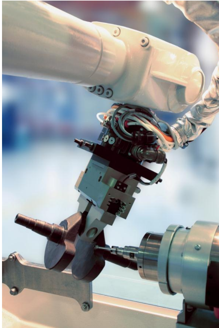
Figure 3 - Radial compliant spindle for the finishing operation of a motorcycle shaft (Courtesy: SIR Spa – MO, Italy).
