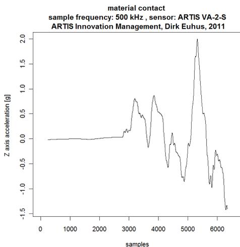
Picture 5) first micro seconds of milling tool contact
