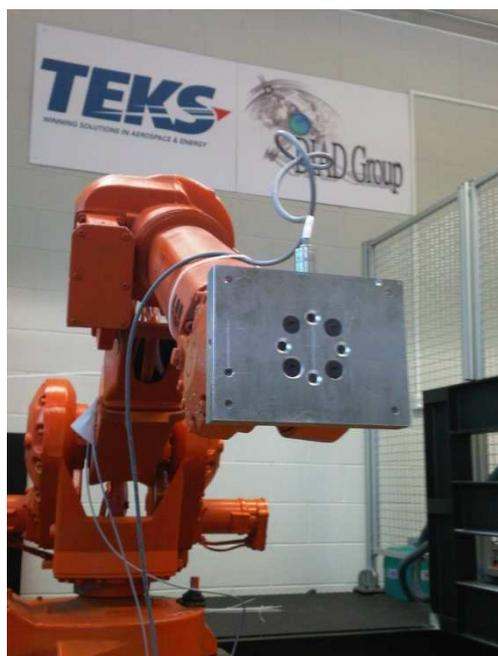
Picture 1) TEKS robot with ARTIS acceleration sensor VA-2-S in Z direction
