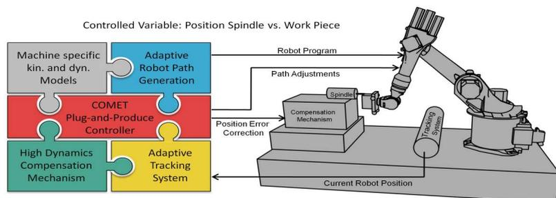
2. The complete COMET platform for high accuracy machining with robots
