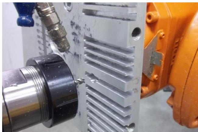
8. Milling slots and the fake hole to simulate a process error
